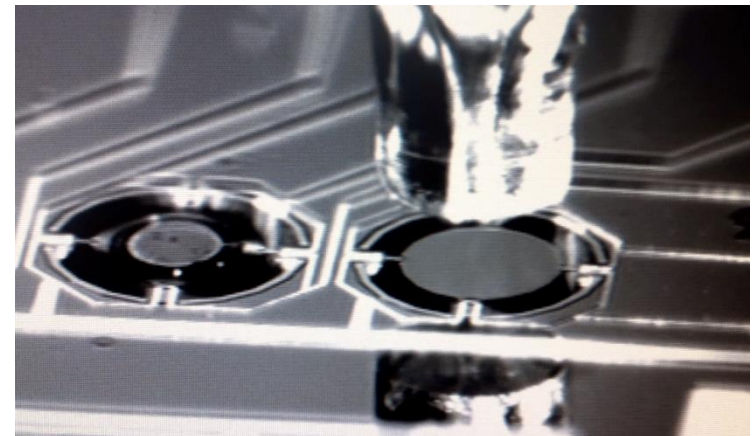
Inkjet spotting for MSS coating e.g. polymers such as PSS, Dextran, CMC, PVP
